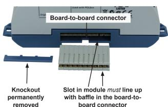
Figure 7: Communication Module with Board-to-Board Connector Inserted
